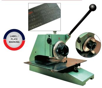
Leaf gauge for multi-line labels. This special leaf-gauge can be custom-built to your individual need. It enables speedy alignment of each lines before marking!. After marking a line, a leaf is flipped for immediate setting to mark in the next line! Stops for 2-lines labels Specially for 2-line marking, there are two stops (supplied with machine) to enables faster, accurate automatic alignment of each line before marking.
