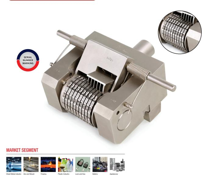
Serial Numbers can be Marked on Metal Parts - in a Simple Operation. Special Design Ensures that Numbers Advance One - at - a Time Accurately and Automatically.
